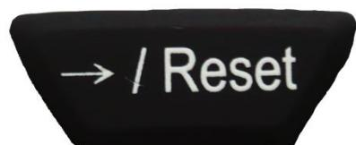
Press [->/Reset] Key for 2 seconds to set number to zero.
