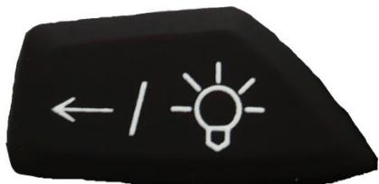
Press Light Sign to turn on the backlight by 2 seconds. The light will turn on 15 seconds then turn off automatically.
