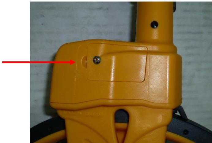
Open battery case by a screw driver.
